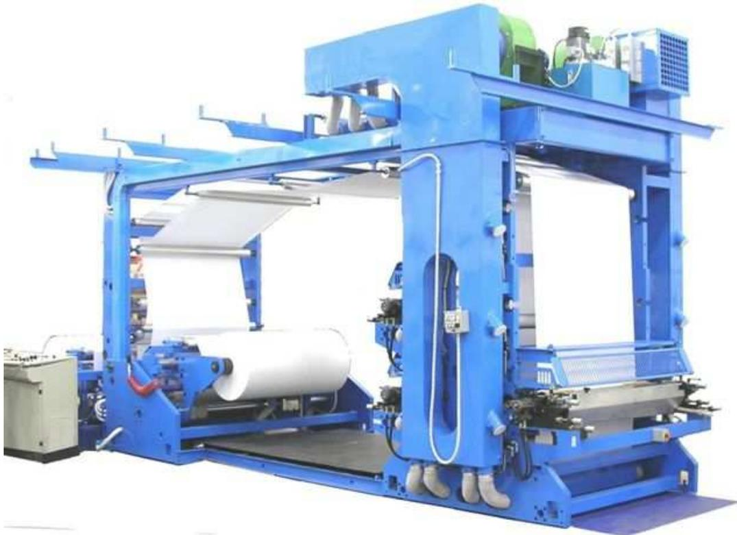
The print-station **Baby-Flex FX** is a stamp system up to 6 colours, from reel to reel, suitable for print water based or solvent base ink on film or on paper, with a max speed of 300 m/min. The Baby-Flex FK has an anilox-ceramic cylinder dia. 127 mm, with doctor blade system. The machine can be equipped of gas burner dryer, side guides, corona treatment, edge cutter, inspection camera, clichè holders, rear-front side print. The machine is available with different type of unwinder/rewinder.
